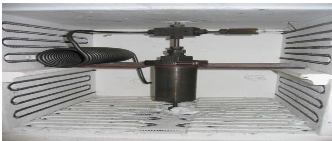
Fig.-1: Supercritical water ethanol reforming experimental setup
